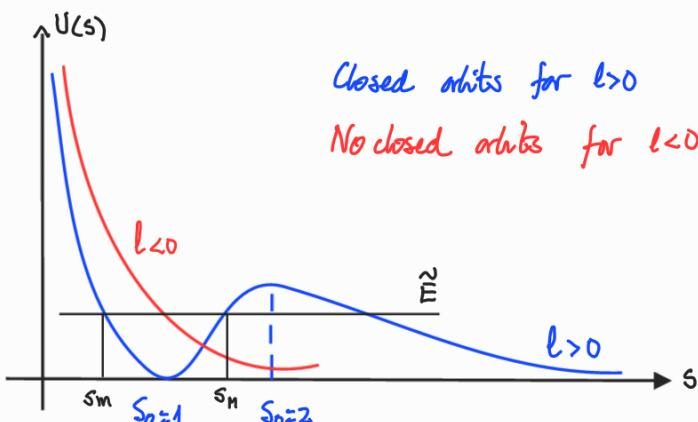
For an energy  $0 < \tilde{E} < U(s_0=2) = \frac{3\ell^4}{32m^2\mu^2g^2}$  there is a closed orbit with periastron  $r_m$  and apastron  $r_M$ .
