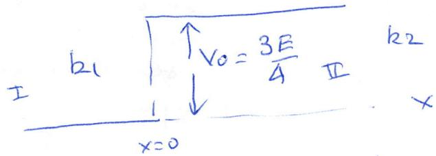
$$k_1 = \sqrt{\frac{2m(E)}{\hbar^2}}, \quad k_2 = \sqrt{\frac{2m(E-V_0)}{\hbar^2}}$$
